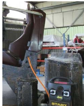
Test Box Connection on Coaster Vehicle
