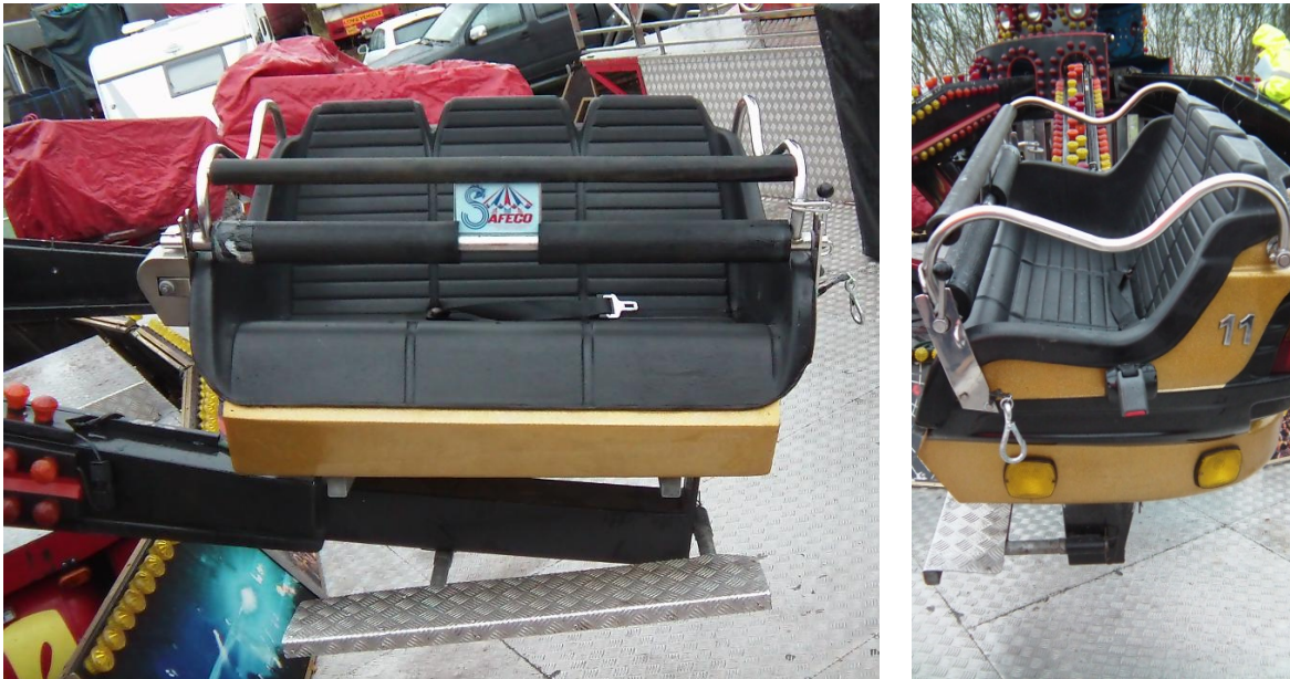
Figure 20 DJ Jump seating and restraint system
