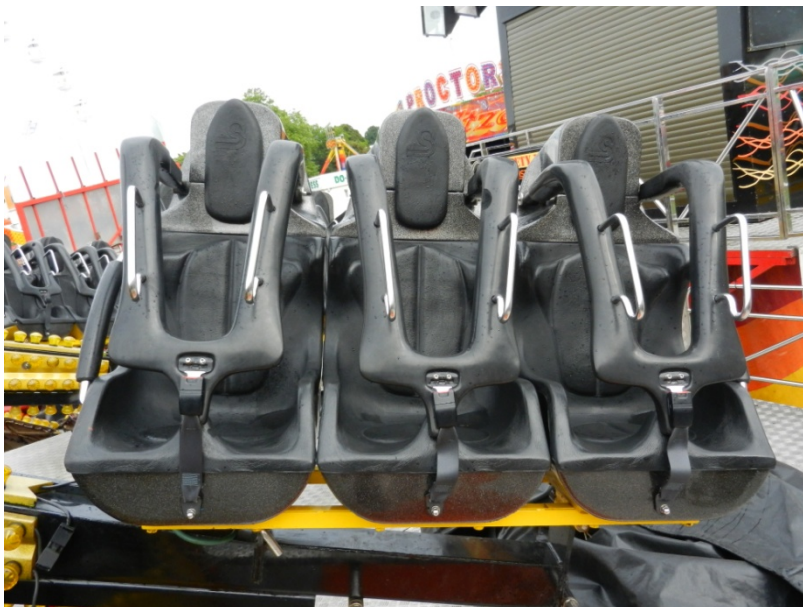
Figure 21 Alternate passenger restraint design
