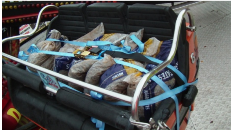
Figure 3 Representative load of 160 kg
