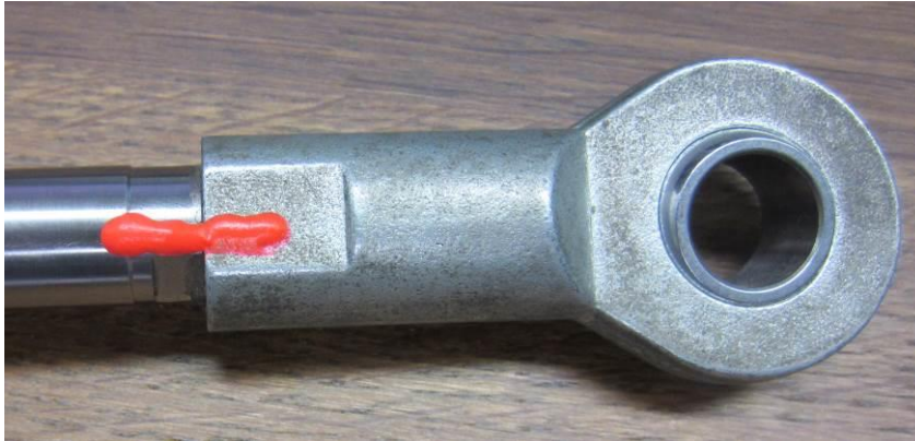
Figure 1: how to apply torque striping on the rod end.
