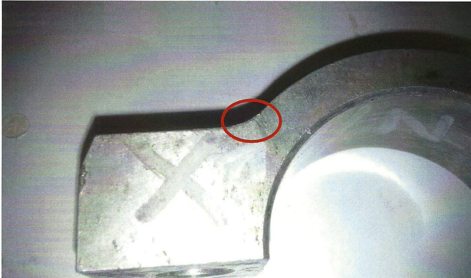
Figure 2 Cracks of bearing blocks
