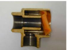
Figure 2 - Floating Piston in misaligned position
