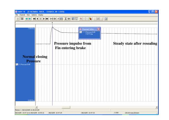
Figure 3. Chart of Pressure Pulse
