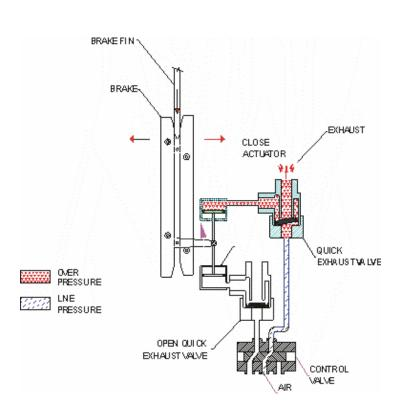
Figure 4 – Quick Exhaust Valve Failure Mode
